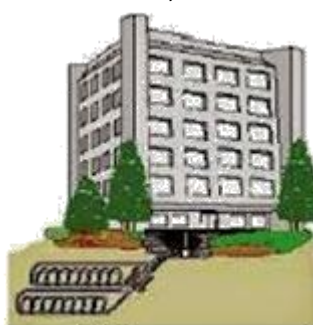
Graphic 11: Horizontal closed loop.
