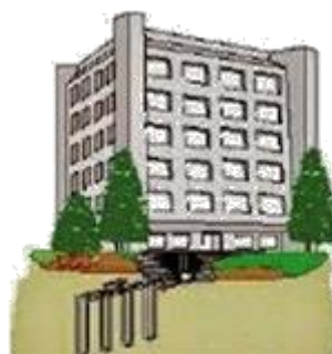
Graphic 10: Vertical closed loop.
